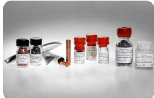
Availability: BCR-098: Bottles containing about 10 g of chips. BCR-275: discs of 13 mm diameter and 1 mm height (+/- 10 discs in bottle)
